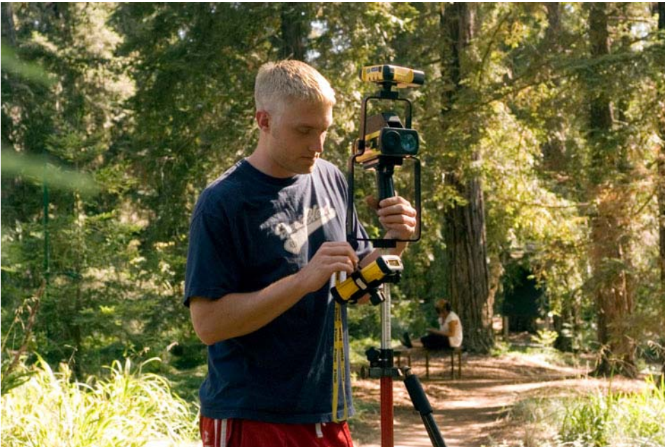
Figure 2. Student teams used GPS equipment to collect latitude and longitude location information for individual plants in the arboretum.
