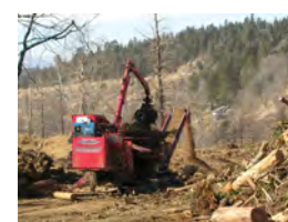
Tubgrinders were used to quickly convert woody debris, logs and whole trees into biomass chips and compost/mulch feedstocks.
