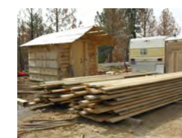
A niche market developed for locally produced rustic siding produced from salvage incense cedar.
